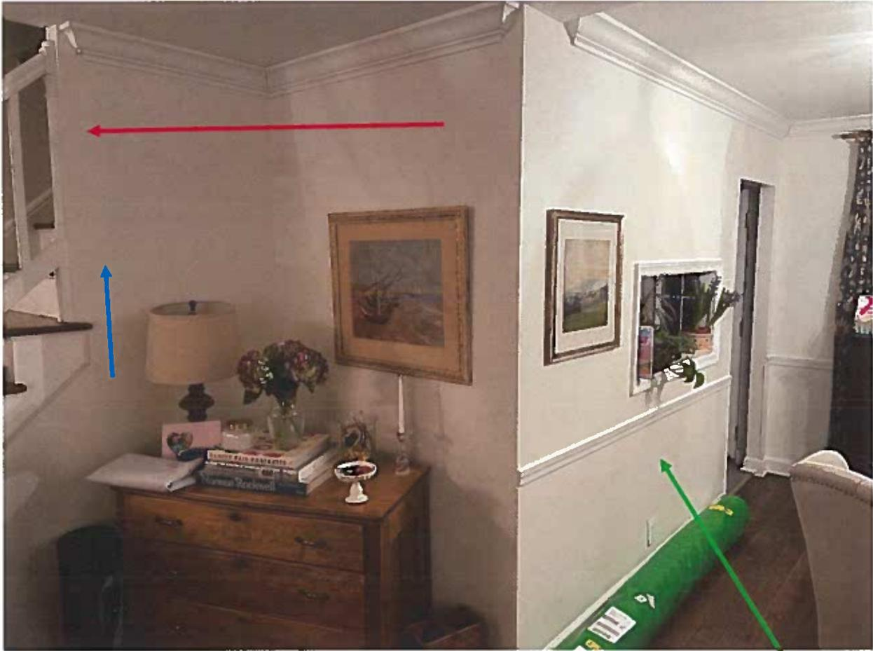
Request to move wall with red arrow to the position of blue arrow and to remove entirely the wall with the green arrow.
